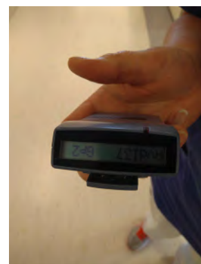
Fig. 232. Hall call device for nurses. They receive calls from designated patients with the room number. SAHLH.
