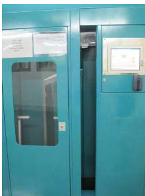
Fig. 7 Automatised system for linen cleaning and delivery. There is no laundry in the acute-care hospital as the service is externalised. Staff have to identify themselves electronically each day and get their uniform. HSCP.
