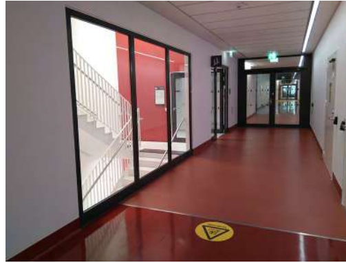
Fig. 95 Pavement signal warning of goods trolley movement from goods lift. NKS.
